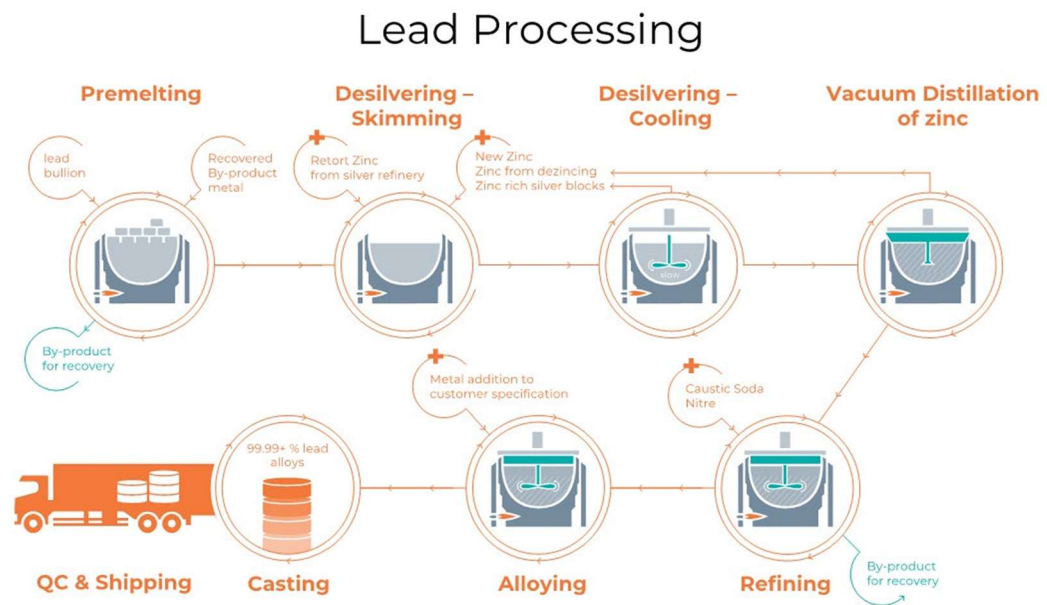
Figure 3: Processing of lead at BRM
